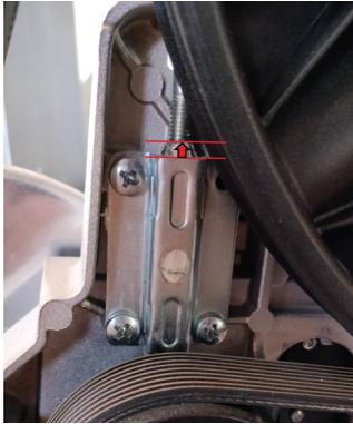
4) Use a 5mm allen key to completely untighten the tension screw and remove the belt.
